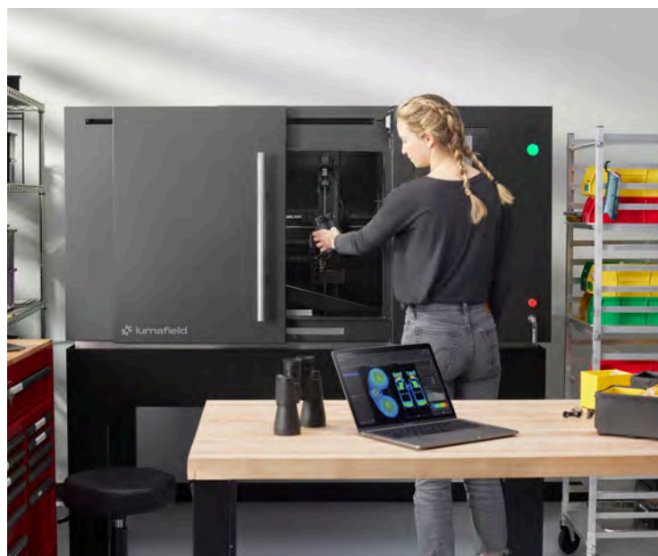
▲ Lumafield's Neptune industrial X-ray CT scanner.
